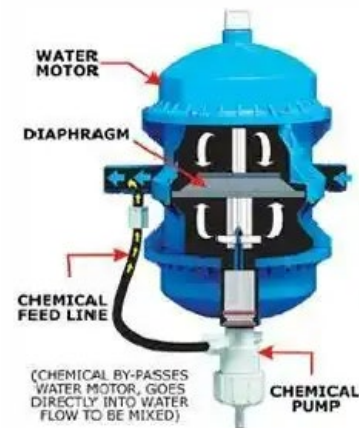
Figures 2.18a and 2.18b. Examples of the Venturi principle injector (2.18a; courtesy of irrigationking.com) and a piston type chemical injector (2.18b; courtesy of Solutiontrade.co.in).
