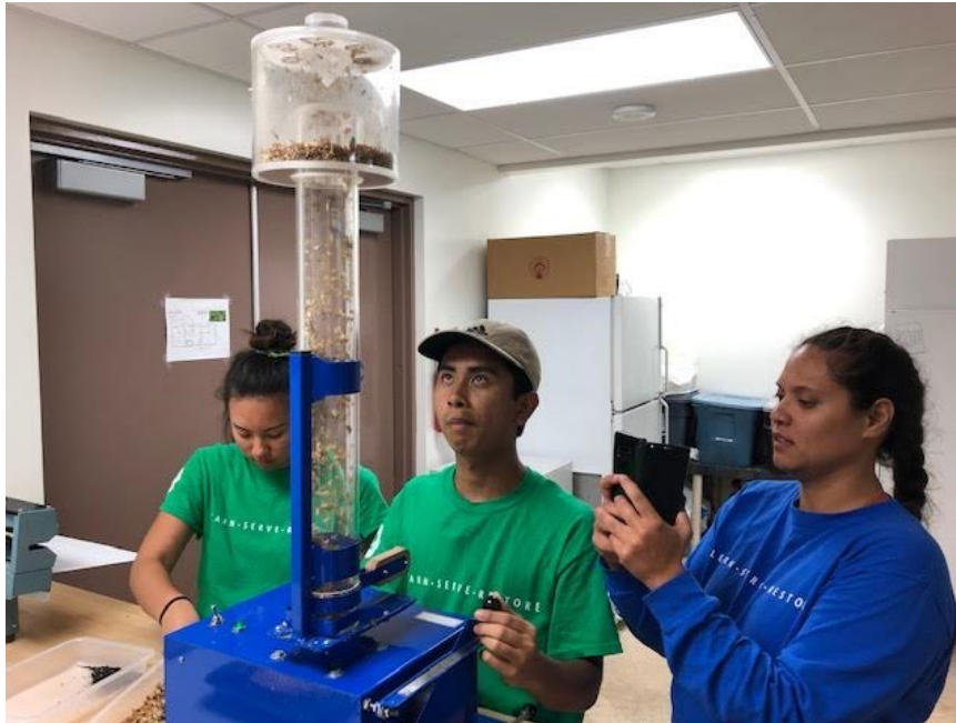
Figure 2.05. The column blower being used to separate Dodonaea viscosa seed from the fruit. The column blower works well for large batches of dry fruits where the seed is significantly heavier than the fruit.
